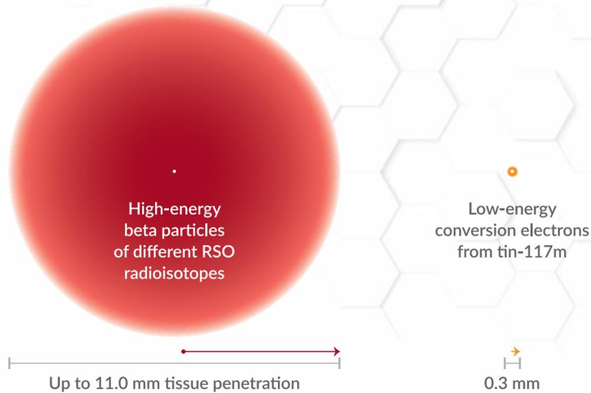
**Figure 1.** The diagram compares the radiation dose range of conversion electrons emitted by tin-117m (300  $\mu\text{m}$ , 0.3 mm) with beta radiation emitted by radionuclides such as yttrium-90 and erbium-169 (up to 11,000  $\mu\text{m}$ , 11.0 mm). The ultra-narrow, discrete radiation range of tin-117m enables more precise dosimetry and avoidance of adverse effects on adjacent tissues such as what can occur with beta-emitting radionuclides.
